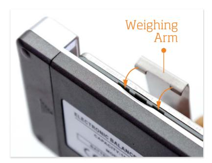
Locate the Arm fixing recesses on the underside of the weighing platform and gently slide the lugs of the weighing arm into the two outer recesses as shown.
