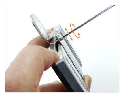
Using the allen key, carefully position and fit one wing of the T-Nut into the middle recess on the otherside by rotating and sliding it into the recess as shown.
